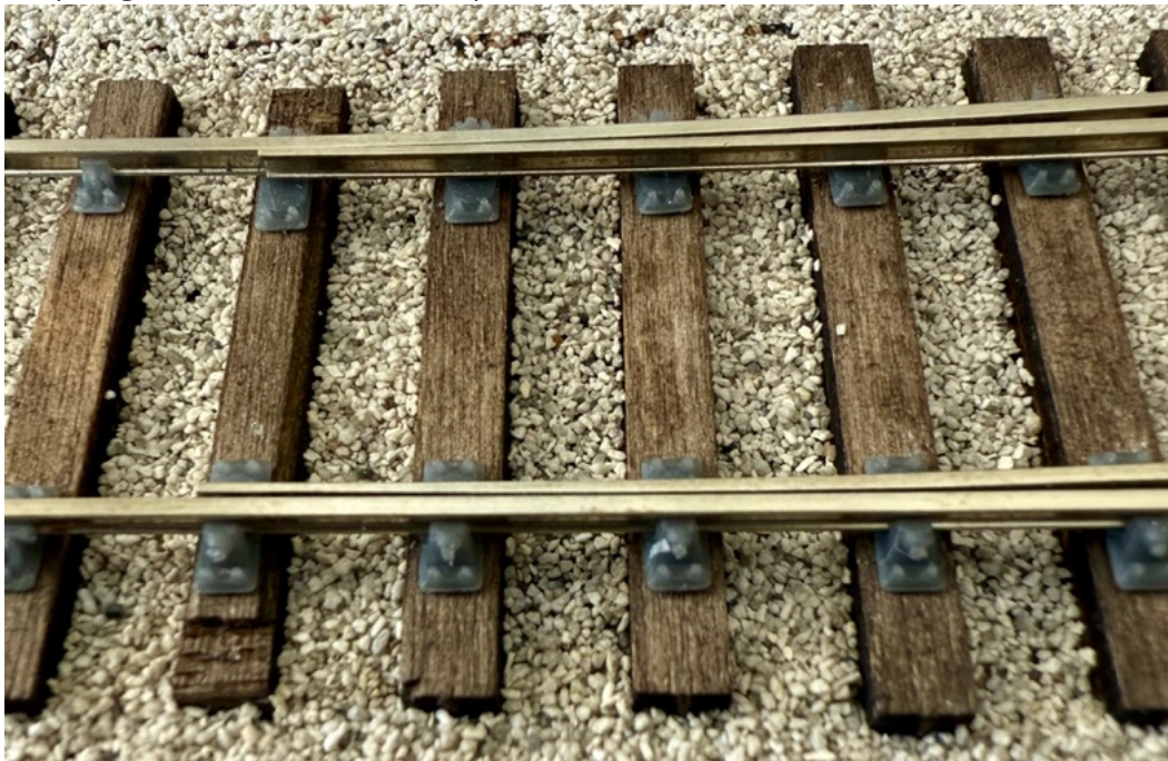
Photo of 4mm 00-SF B7 switch blades filed using back of blade filing jig.
