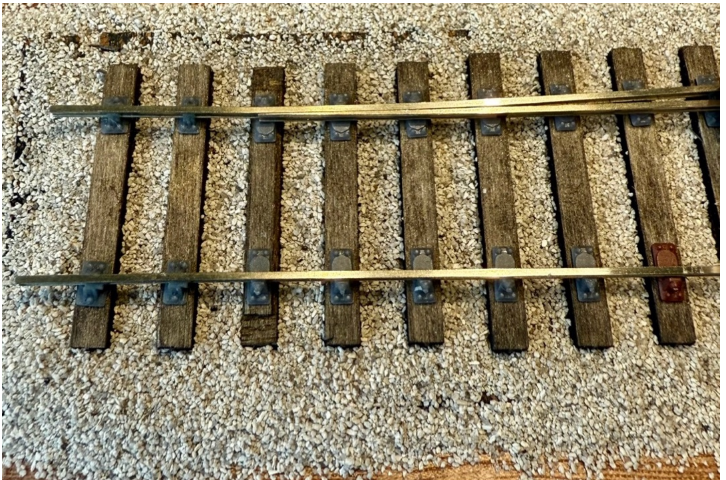
Photo of 4mm 00-SF B7 switch blades filed using back of blade filing jig & front head rail at 20 °
